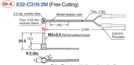
Note: There is a white line on the emitter fiber. M3 nuts (Nickel-plated brass) Washers (Nickel-plated brass) provided (2 of each)
