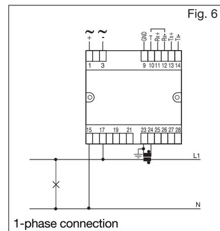
**NOTE:** Only for “PG” and “SG” options: the current measuring inputs are galvanically insulated and therefore they can be connected to ground singly.
