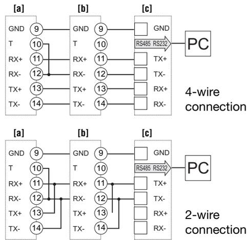
Fig. 7: **a**-Last instrument; **b**-1...n Instrument
